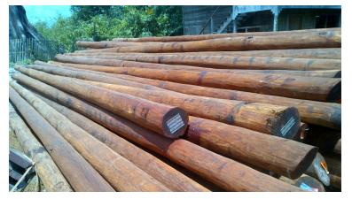
This natural wood has a "Class A" fire rating, making it almost as fire resistant as metal or concrete. With an incredible resilience and life span of over 50+ years, Wallaba posts and poles can save time and money by avoiding costly repairs and replacements.
