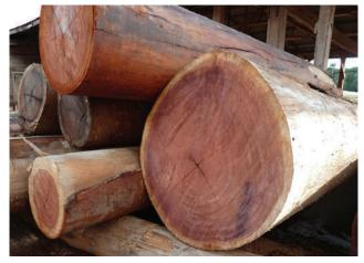
weathering elements. Kiln drying is also available but not necessary unless the materials are going to be used indoors where artificial heating and cooling are utilized. We evaluate each of our customer's project locations and determine the best drying application.
